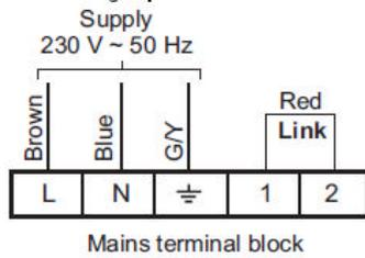
**THREE WAY VALVE CONNECTIONS**
